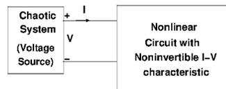
Fig. 6. Scheme of a nonlinear system where a chaotic voltage source is used as the input signal for a nonlinear circuit with a noninvertible  $I$ – $V$  characteristic.
