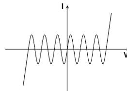
Fig. 5. Noninvertible  $I$ – $V$  characteristic. Many extrema.
