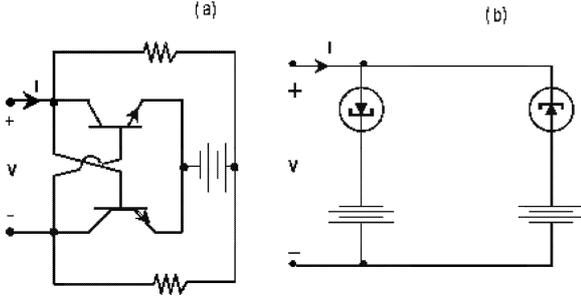
Fig. 7. Nonlinear circuits with noninvertible  $I$ – $V$  characteristics. (a) The resistors possess  $R = 2.2 \text{ k}\Omega$ , the source voltage in the battery is 10 V and the twin transistors are 2N2222 with  $\beta = 140$ ). The  $I$ – $V$  characteristic of this circuit is shown in Fig. 4. (b) Another circuit with a similar  $I$ – $V$  characteristic.
