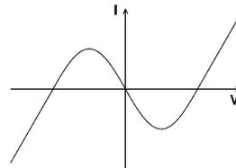
Fig. 4. Noninvertible  $I$ – $V$  characteristic. Two extrema.
