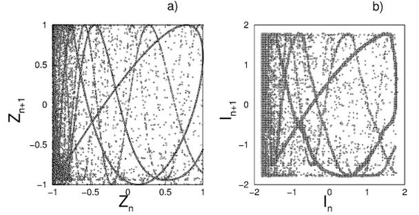
Fig. 8. Modelling versus experiment. (a) Numerical simulation of the dynamical system (23)–(25); (b) first-return map produced with the real data (current measurements) from experiments using the scheme of Fig. 6, where the circuit of the right is the one of Fig. 7(a).
