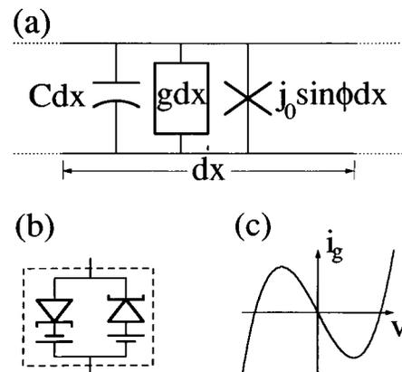
FIG. 1. Active transmission line. (a) Element of the lumped transmission-line circuit;  $1/g$  is the nonlinear resistance. (b) Negative resistance twin-tunnel-diode circuit. (c) Nonlinear characteristic of the negative-resistance oscillator.
