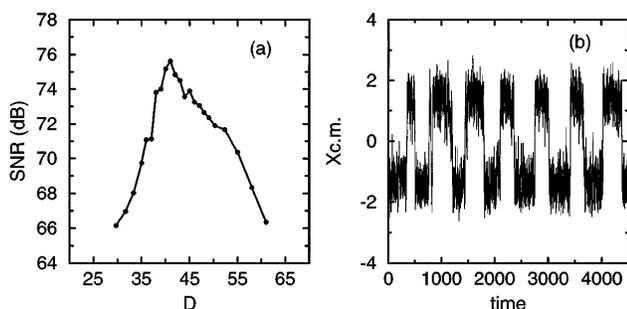
FIG. 2. Two aspects of the solitonic stochastic resonance: (a) There is a maximum of the SNR at a critical value of noise intensity. (b) Synchronization of the stochastic jumps with the periodic perturbation linked with translational mode of the soliton. ( $P_0 = 0.04$ ,  $\omega = 0.01$ ,  $x_0 = 2.5$ , and  $B = 0.7$ .)
