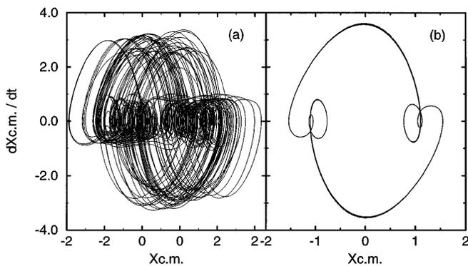
FIG. 1. Phase portraits for the motion of the soliton center of mass in Eq. (7);  $F(x)$  is defined as in Eq. (2) ( $B = 1/2$ ). (a) Chaotic motion in the absence of control [ $F_c(x, t) \equiv 0$ ],  $\gamma = 0.1$ ,  $A = 1.5$ ,  $P_0 = 1$ , and  $\omega = 0.65$ . (b) Periodic motion as a result of the application of nonfeedback control,  $\omega_c = 0.065$ ,  $g_c = 0.35$ , and  $\theta_c = 0$ .
